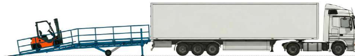
In the absence of a loading dock, the ramp connects the "Ground-Machine" levels.
